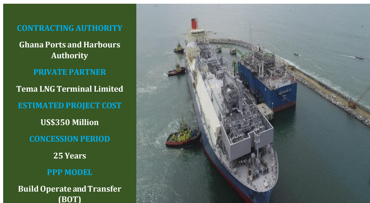
Figure 11: Floating Storage Unit (FSU) and Floating Regasification Unit (FRU)
