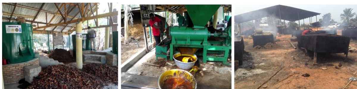
Improved cookstoves with chimneys, Steamers and clarification tanks to replace traditional cooking stoves
