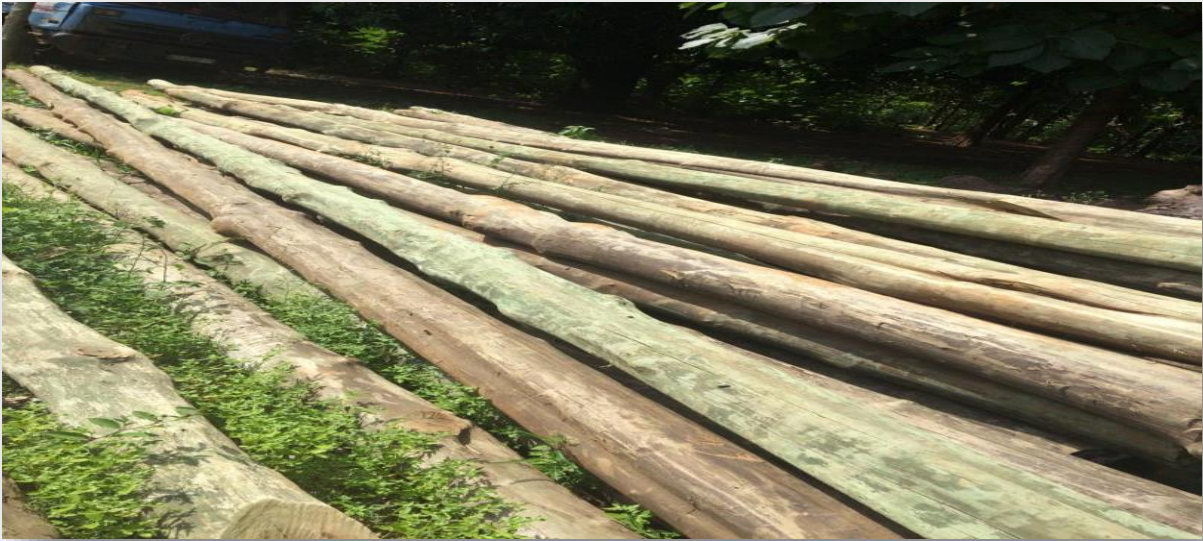
Figure 11: Procured and distributed 100 No. 9 meter Low Tension Electric Poles
